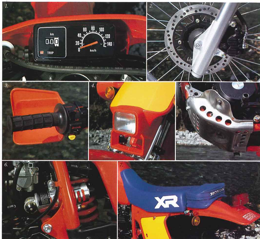
1. Large-dial speedometer with easy-read, easy-set tripmeter. 2. Lightweight disc brake with dual-piston caliper (XR250R). 3. Compact, convenient switch location. 4. Rectangular high/low beam headlight. 5. Large, lightweight, aluminium skidplate. 6. Pro-Link suspension with remote reservoir. 7. Seat-over-tank design and tough, zippered tool pouch.
